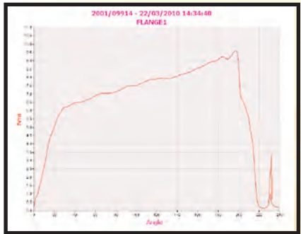
Torque vs Angle graph produced using TDMS software
