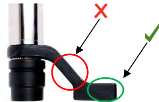
FIGURE 6 – Cranked Reaction Bar (Steel or Aluminium)
